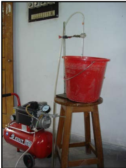
Fig. 1. Volume flux per plant (F A[-] ), measurement using aspirator in excised rice root at submerged condition in a bucket.
